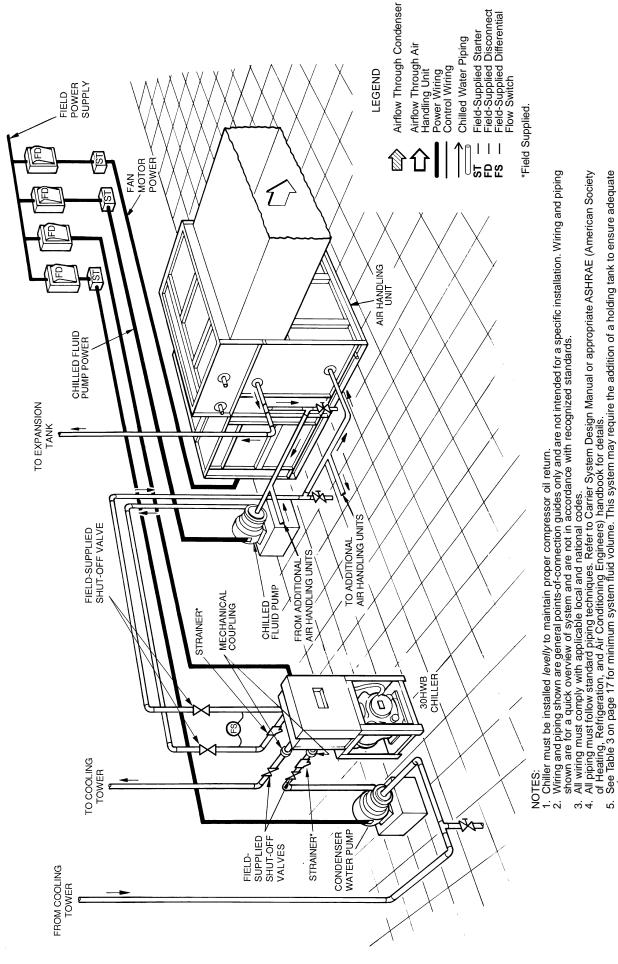
Fig. 13 — Typical Piping with Fluid-Cooled 30HWB Unit Shown
